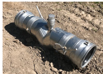
Riser for poly pipe to attach to
